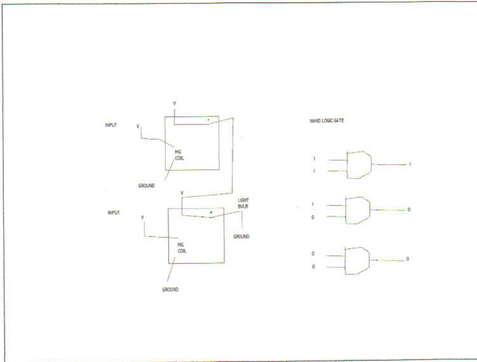
If we rewire the connections between the two coils, as above, and vary the input values in order to get a Boolean valued output, then the total system represents what we now call a NOR logic gate.
