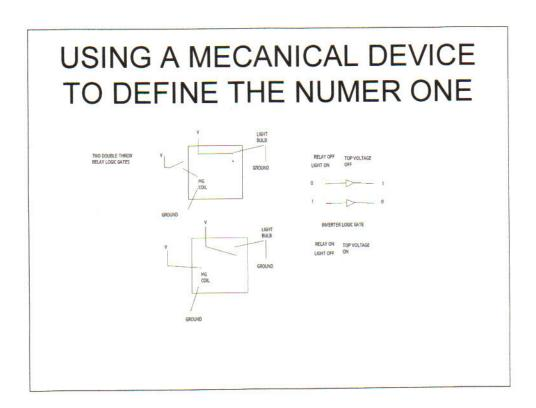
USING A MECHANICAL DEVICE TO DEFINE THE CONCEPT OF THE NUMBER ONE
